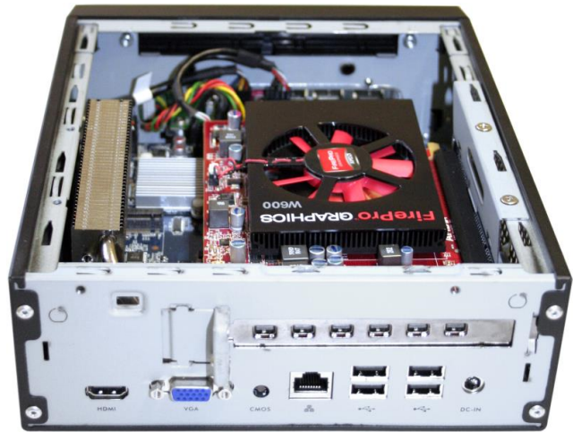
Image: Shuttle XPC slim Barebone XH110G with built-in AMD FirePro W600 graphics card
